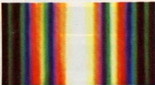
B. Passing white light through a single slit produces this diffraction pattern.
