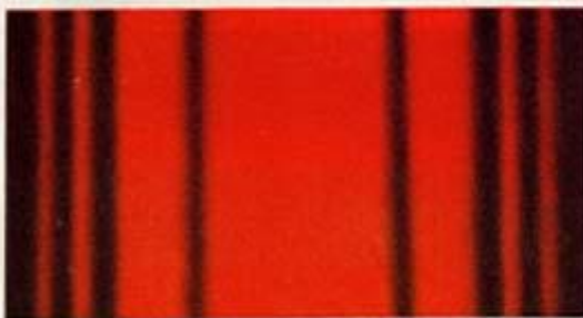
Red light passed through the same slit produces this pattern.
